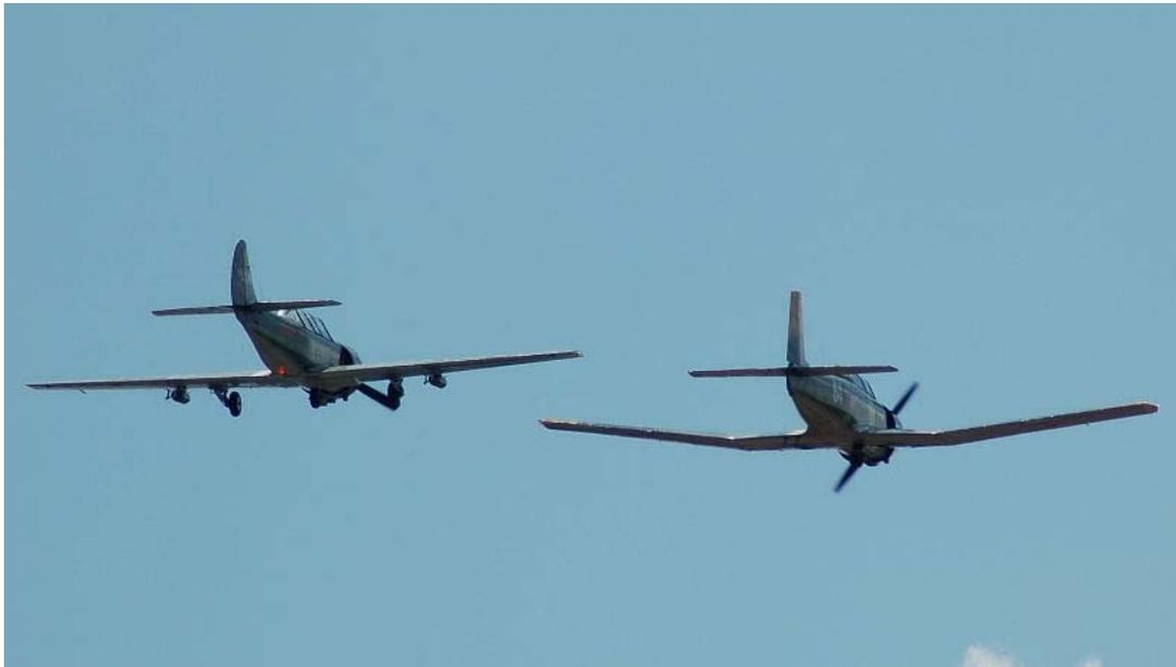
YAK-52 on left and CJ-6 on right. Note the difference in wings. Also note the CJ main landing gear retracts fully into the belly as does a YAK-52TW. The “Straight” YAK main landing gear remains partially extended although retracted.
